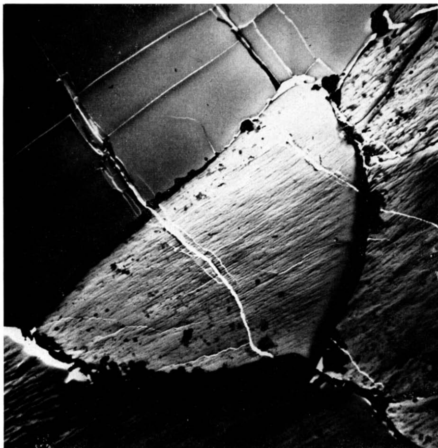
Fig. 1. Lincoln wool fibre, untreated. Direct (negative) surface replica (SiO). Photographic print from original micrograph. \times 10,000 .
