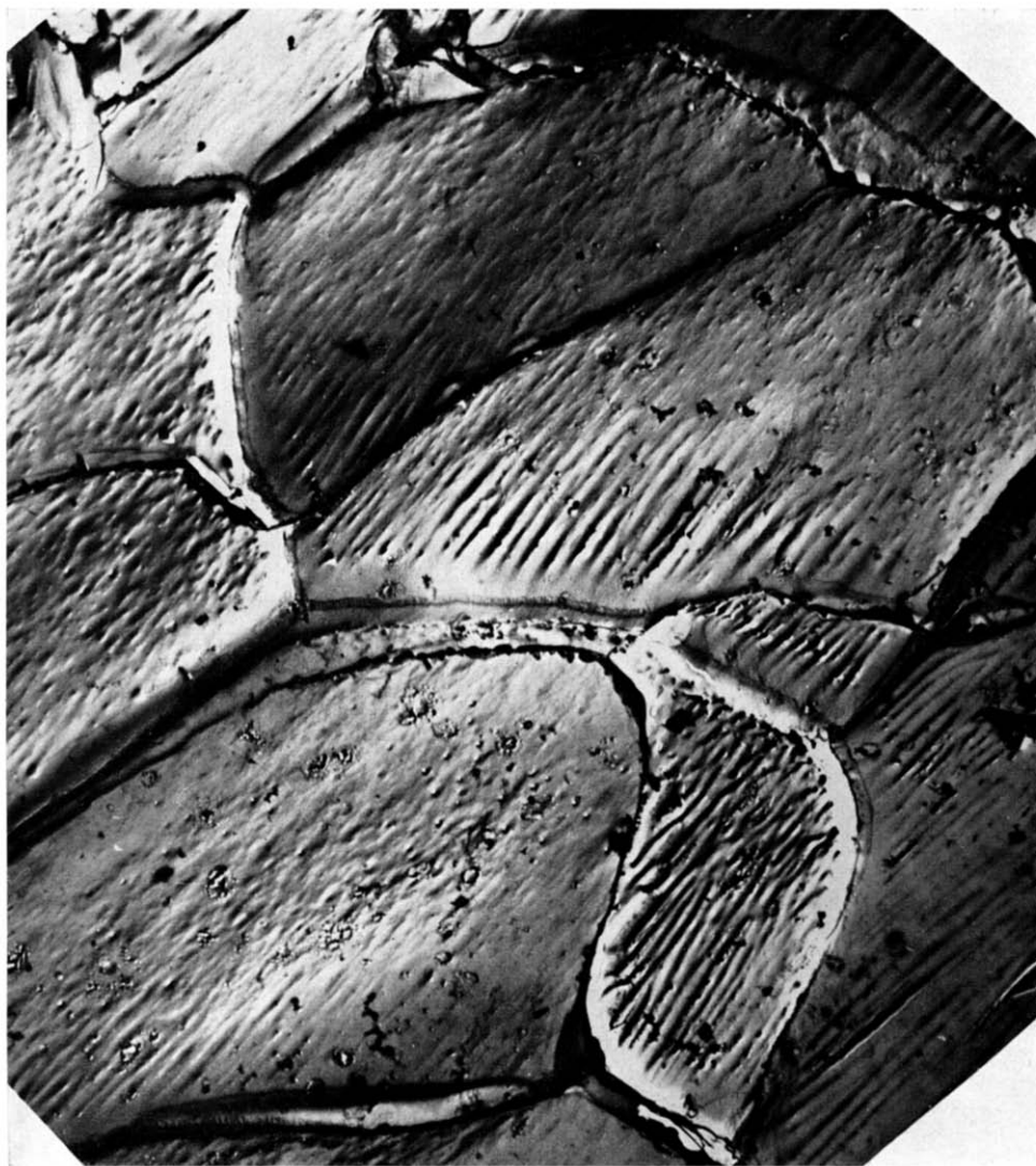
Fig. 3. Lincoln wool fibre, untreated. Two stage (Ag/SiO) surface replica. Photographic print from original micrograph. \times 4,600 .
