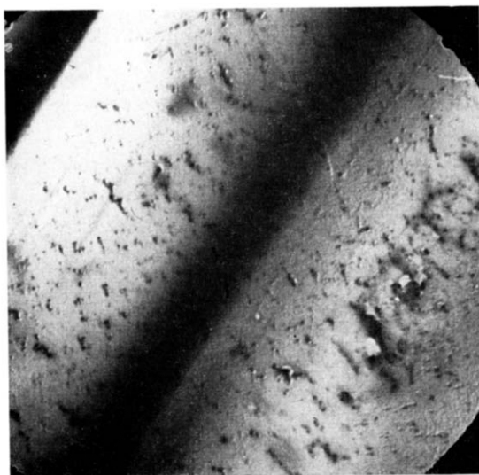
Fig. 13. Acetate rayon fibre, stretched to breaking point. Direct (negative) surface replica (SiO). Photographic print from original micrograph. \times 4,000 .
