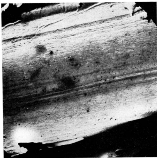
Fig. 14. Raw silk fibre. Direct (negative) surface replica (SiO). Photographic print from original micrograph. \times 5,600 .
